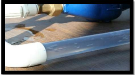
Figure 6 - Clear Pipe Showing Bubbles in the Water Line
